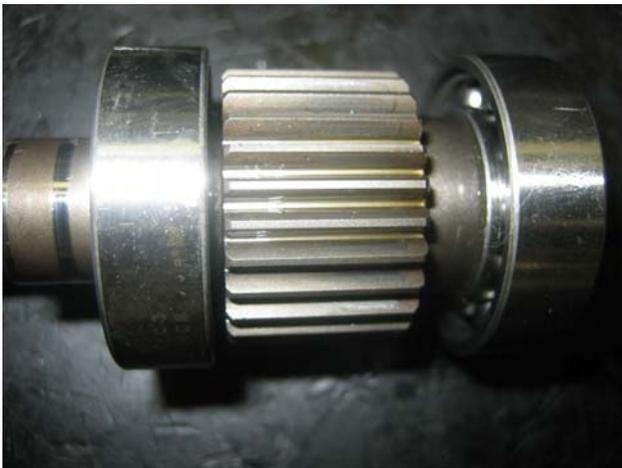
Extremely tight clearance between output gear and bearing.
