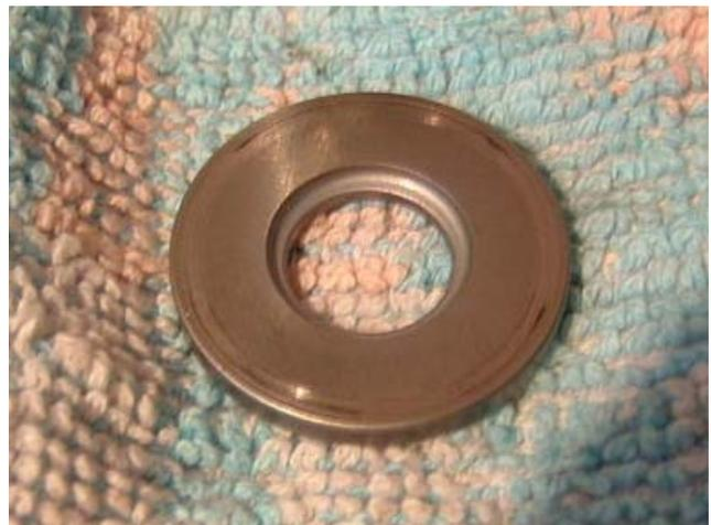
The spacer or washer on the SQ is different, it does not have a chamfer on it. However, it does have a groove in it that faces down toward the gear case.
