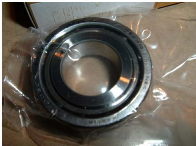
To orient the high speed bearing is very, very easy. The outer race on the thrust side of the bearing will be thicker, that side should face outward or away from the gear. So both bearings thrust sides outward. You will see this on your [supercharger manufacturer] bearings when you disassemble, they will say thrust on that side facing out. So another way to put it is the thicker side thrust side of the bearing will face down into the bearing cups on the gear case and the cover.
