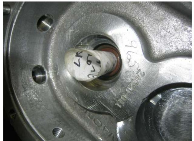
An expansion cone is necessary to insert the shaft without causing damage. I suggest using something flexible and sturdy such as manila, very thin cardboard, or card stock.
