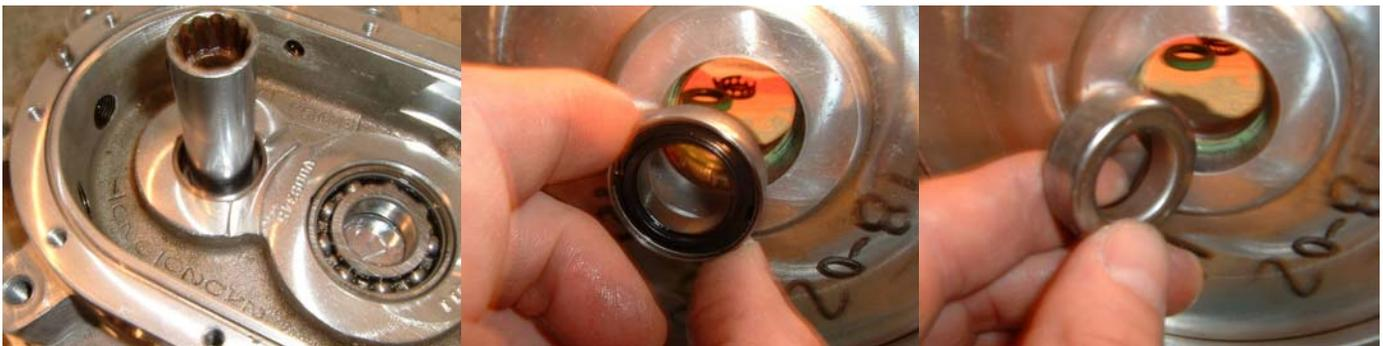
Here is a pic of the seals as you can see they are not Chicago rawhide seals they are SKF. I gave the parts guy the Chicago rawhide part #'s 9776 and 6428 listed by NotoriousNotch. When they arrived they were SKF brand. I was told that Chicago rawhide is now SKF and most seal and packaging has the SKF logo and new parts numbers as you can see by the boxes.
