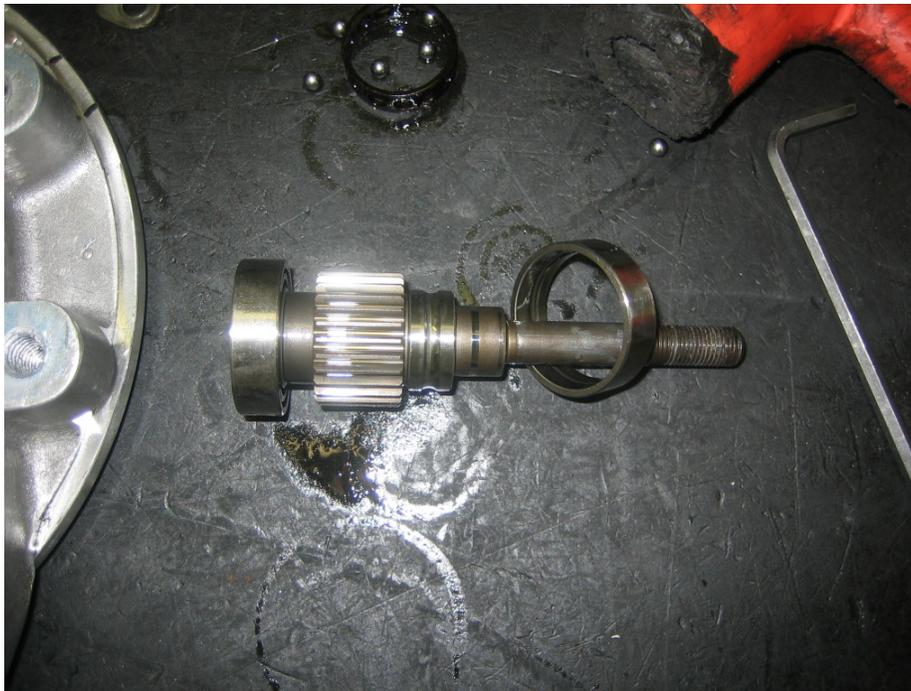
Here's what you're left with if you're not careful, note the ball bearings everywhere! A busted bearing and an inner race that's still on the shaft. No big deal if you're going to replace the bearings.
