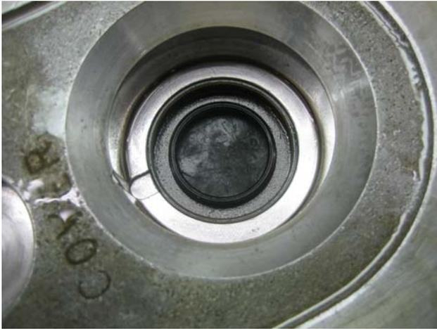
Input seal can be removed with a socket that fits between the ID and OD.
