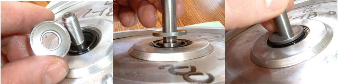
Another noted difference in the SQ is the cover to the impeller has an orange gasket (seal) and a small lip for it to fit into, see below:
