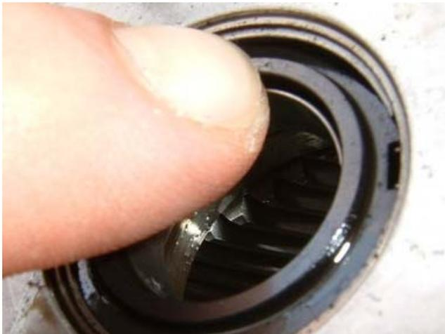
Look how the output shaft seal is hard plastic and pivots. It's spring loaded, there is no soft rubber lip at all.
