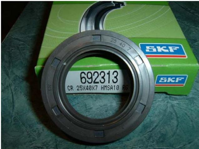
This is the new double lipped SKF seal for the input shaft
