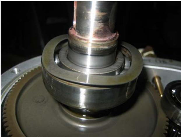
Wave washer for input shaft.
