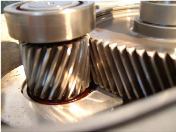
It also appears there is a different style seal for the output shaft, it has a metal in ring that has a hard plastic outer seal that is spring loaded. The plastic part seems to make a seal with the spacer that is between the impeller and the outer gear case. This is not at all like the v-1 units.
