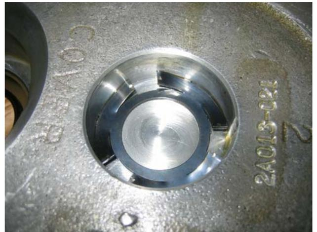
Wave washer for output shaft.
