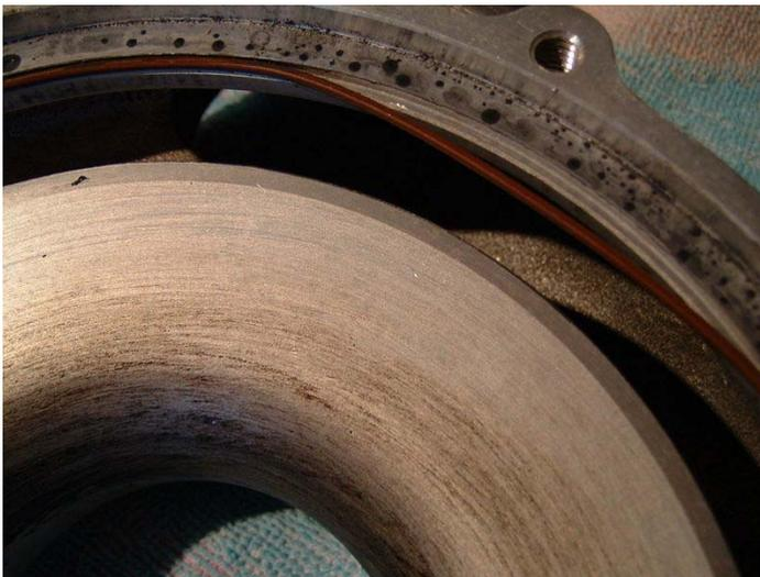
The output shaft seal (compressor seal) was hard to get out. I could not do it with the rubber hammer. I used the press and even that took a lot of force. Remember, this is a different seal than the others (for the V1) seen before.
