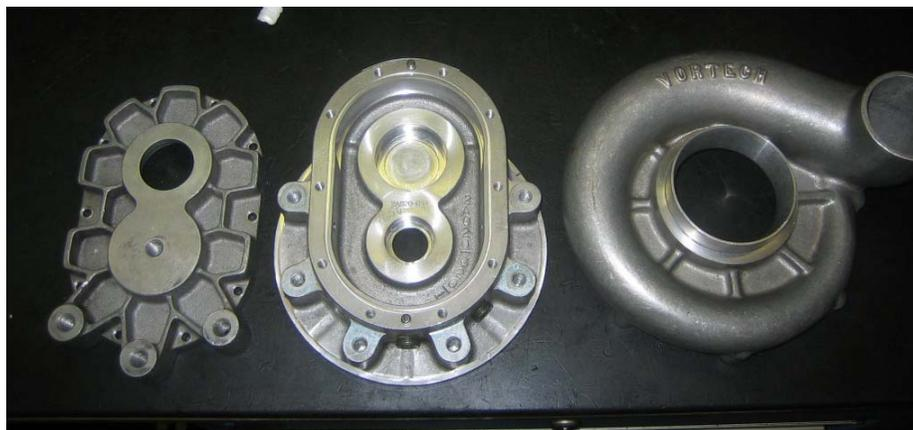
Front cover, gear case, and compressor housing
