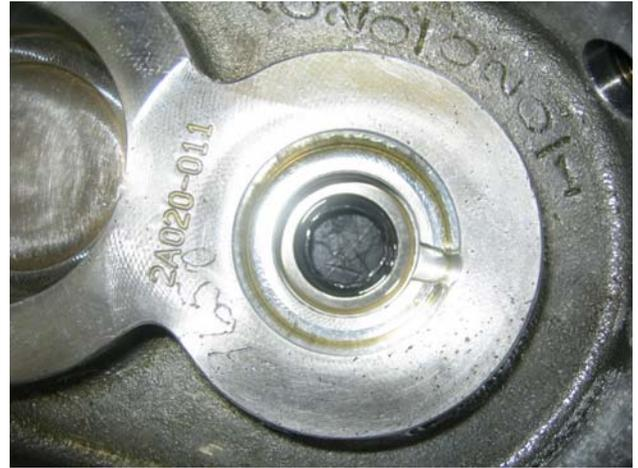
Compressor seal can be removed with a socket that is just larger than the black portion of the seal. The first “inner ring” of metal is actually part of the seal.
